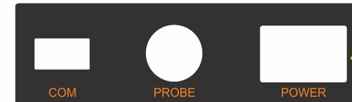
The AC power connector jack is located on the rear panel. The AC power jack is a three-prong, international-style IEC inlet. The AC power supply is fused inside as there are no user serviceable parts inside/outside and a blown fuse will require attention qualified personnel from the company. The unit is not supposed to be reused with a fuse from outside for safety reason. The AC type i.e. 115 or 230V 50/60Hz is indicated on a sticker on the left side of Hot Plate.
